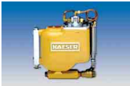
Kaeser's AMD 6550 is designed for "no loss" operation on larger filters and vessels. It uses a magnetic actuator that is isolated from the contaminant chamber so the drain does not stick open or closed. This heavy duty drain has a four year warranty and requires no electricity.
